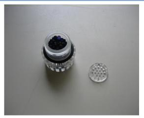
Exchange the desiccant then put the inner lid back on the cartridge. Place the drying cartridge back on the MS-57 body and secure it gently.
