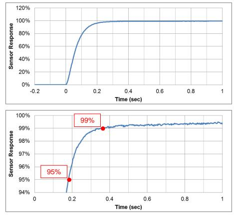
Figure 7-2. Response Time Measurement
