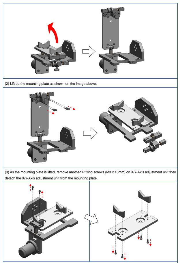
(4) Remove 2 fixing screws (M3 x 15mm) for mounting plate. Detach the mounting plate from the Sun Tracker Arm, and remove the fixing screws on both V-Blocks (M3 x 5mm in 2 places on each V-Block).
