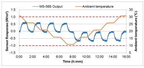
Figure 7-4. Zero Offset Measurement
