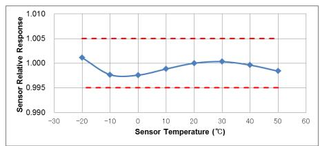
Figure 7-3. Temperature Dependency Measurement
