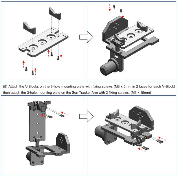
(6) Attach the X/Y-Axis adjustment unit on the 3-hole mounting plate with the fixing screws (M3 x 15mm in 4 places) then attach the X/Y-Axis adjustment unit on the Sun Tracker Arm with the fixing screws (M3 x 15mm in 4 places)
