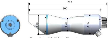
Figure 7-1. MS-57 Outer Dimensions
