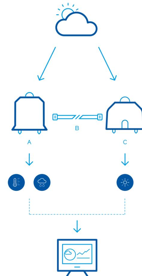
On the left: the new ASI-16 imager can now be connected to the compact MS-80, combining measurements of temperature, humidity and irradiance.
