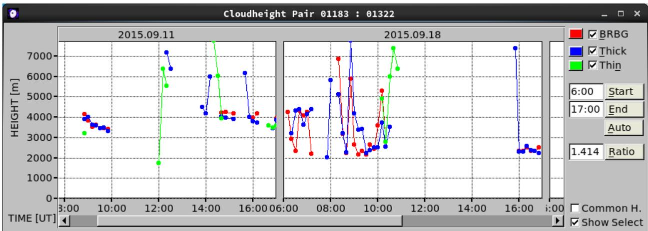
This dialog shows the daily evaluation files (e.g. "cloudheight\_01183\_01322\_20150911\_brbg.txt") as graphical line plot, to provide a better overview of changes in the cloud height.
