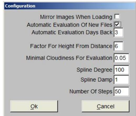
**Automatic Evaluation Of New Files:** When this check box is activated, the software checks all evaluation directories of the current date for new images and evaluates them automatically, when a pair is complete.
