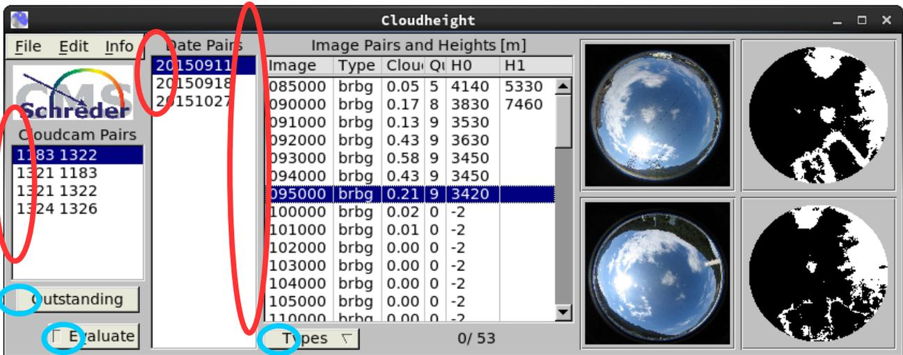
Through the main window it is possible to select the images for evaluation. It shows the results of evaluation, the original images and the "intense-mask" of the images.
