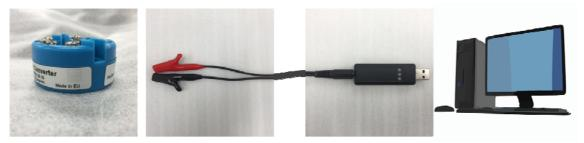
Figure A-6. Connection for Configuring the Signal Converter
