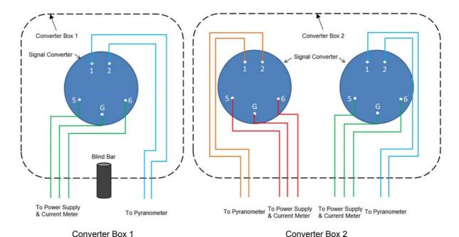
Figure A-22 Wiring Example of Converter Boxes
