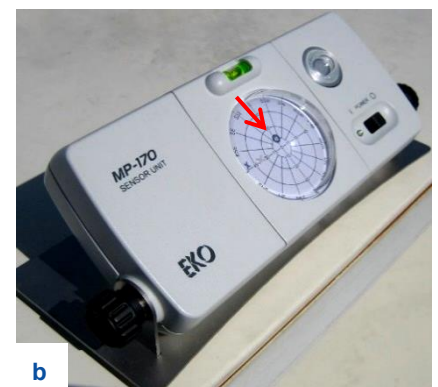
Place Angle Capturer on the Sensor Unit and adjust the position so the shade mark is in the same position as recorded. Figure 5-8. Sensor Unit Installation
