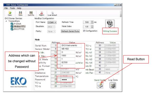
Figure 6-11. Configuration Window (Entering Password)
