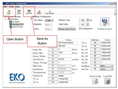
Figure 6-14. Saving and Reading Settings
