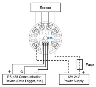
Figure 5-3. Wiring Example
