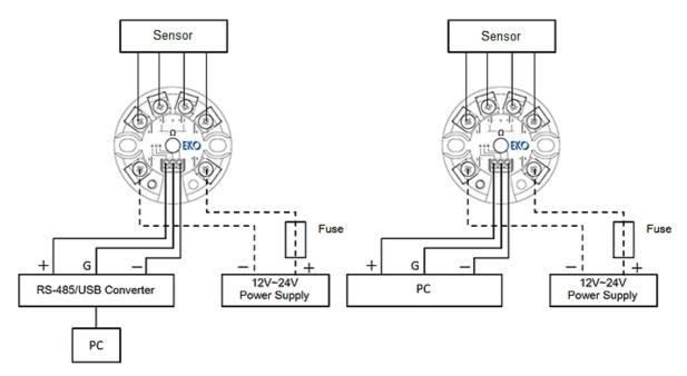
Figure 6-6. Wiring for Converter Setting
