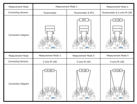
Figure 5-4. Measurement Mode and Measuring Device Connection Terminals
