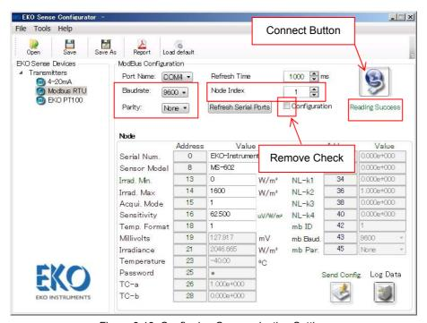
Figure 6-13. Confirming Communication Setting
