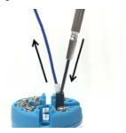
Figure 5-2. How to Remove Communication Cables
