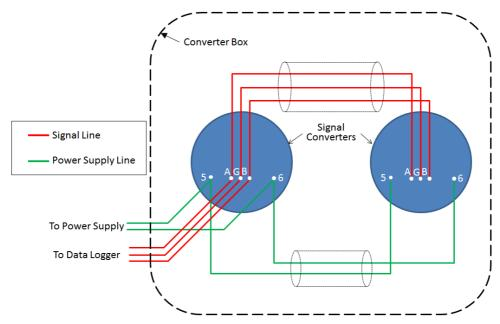
Figure A-4. 2 units of Signal Converter in Converter Box2:
