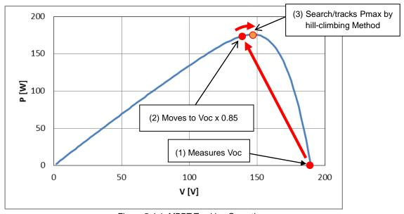
Figure 5-4-1. MPPT Tracking Operation
