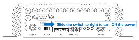
Figure 5-2-6(c). Turning ON the Power
