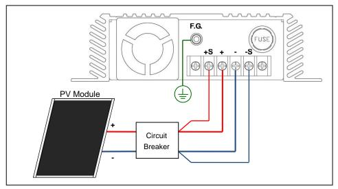
Figure 5-2-2(a). Connecting to PV Module (In-case of 4-wire method)
