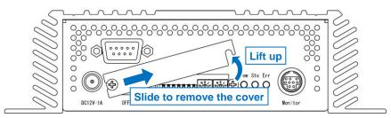
Figure 5-2-6(b). Removing Panel Cover 2
