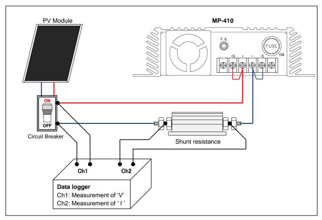
Figure 5-2-3(b). Voltage & Current Measurement Setup (In-case of 2-wire method)
