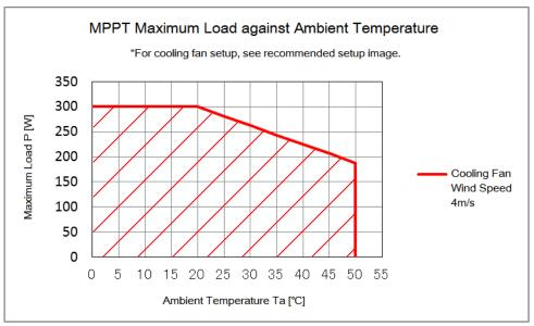
Figure 7-3-1. MPPT Maximum Load against Ambient Temperature
