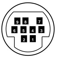
Figure 5-2-4. External Input & Output Control/Monitor Terminal: Terminal Numbers
