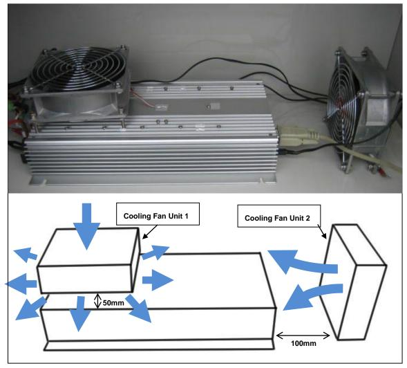
Figure 5-2-1. Recommended Setup for MP-410
