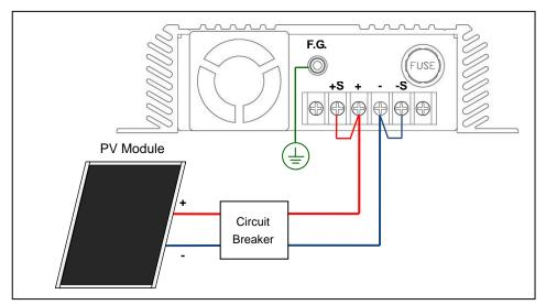
Figure 5-2-2(b). Connecting to PV Module (In-case of 2-wire method)
