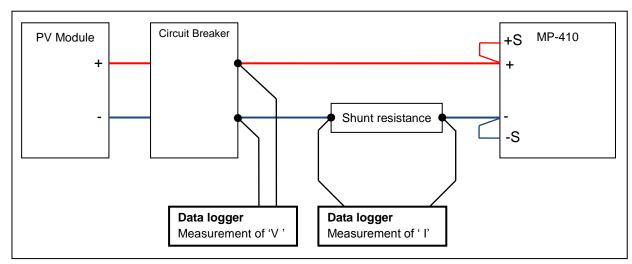
Figure 5-2-3(a). Voltage & Current Measurement Setup (In-case of 2-wire method)
