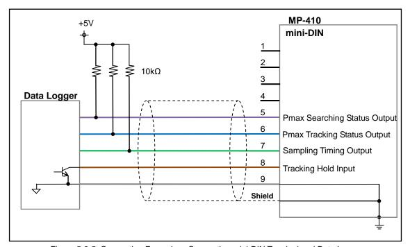
Figure 5-2-5. Connection Example: Connecting mini-DIN Terminal and Data Logger
