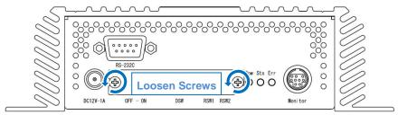
Figure 5-2-6(a). Removing Panel Cover 1
