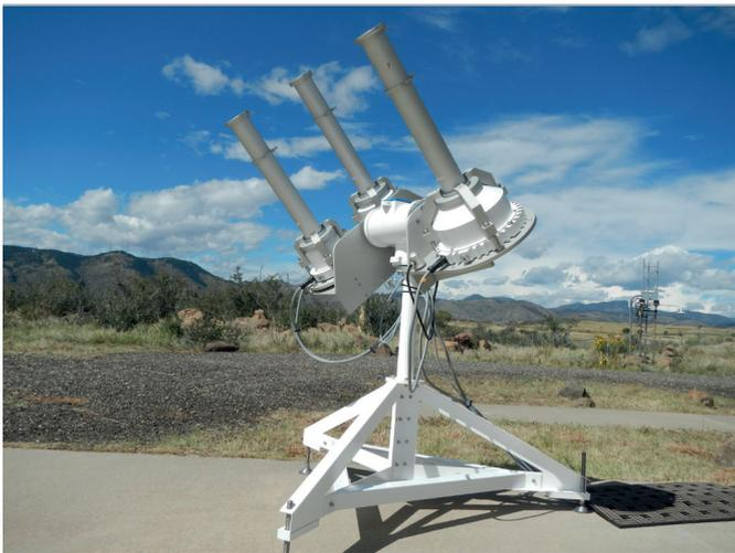
The WISER I is a research-grade configuration, combining the MS-711 and MS-712 Spectroradiometers. A reference tool for UV-VIS-NIR measurements, the WISER I covers the spectral range from 300nm to 1700nm and is designed for meteorological, plant science, photovoltaic research, and material analysis applications that require the highest standards of accuracy and reliability.
