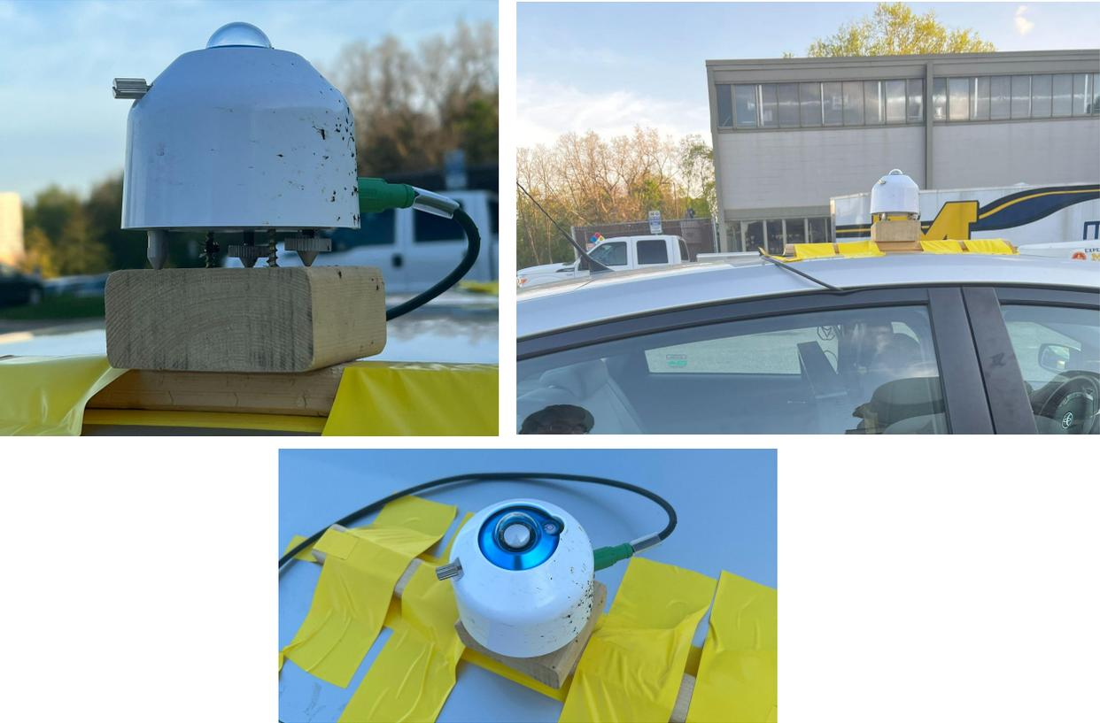
**Figure 4.** Image of MS 80S outfitting for Route Survey
