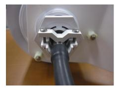
Figure 4-6. Enlarged Image of Inserted Temperature Sensor
