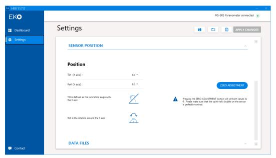
Figure A3-18. Sensor Position setting
