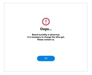
Figure A3-23. Sensor internal humidity abnormality alert
