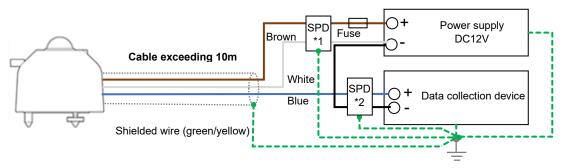
Figure A10-2. SDI-12 connection (when the cable length exceeds 10m, etc.)
