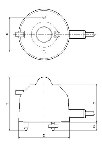
Figure 7-1. External Dimensions (MS-80/80S)
