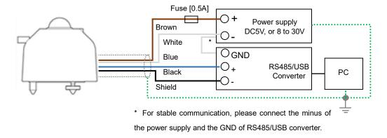
Figure 5-10. How to connect MS-80S (Modbus RTU)
