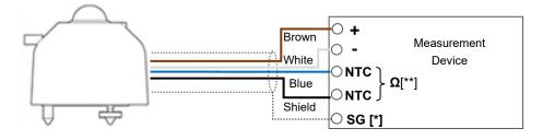
Figure 5-6. How to connect MS-80 (Till S/N: S19046150)
