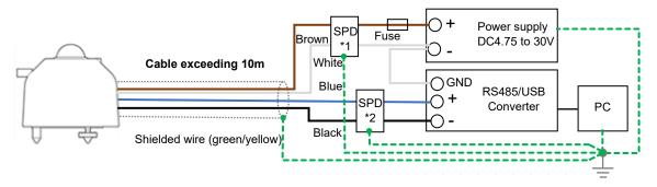
Figure A10-1. Modbus RTU connection (when the cable length exceeds 10m, etc.)
