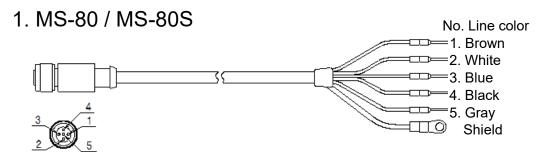
Figure 7-3. Output Cables [MS-80 / MS-80S]
