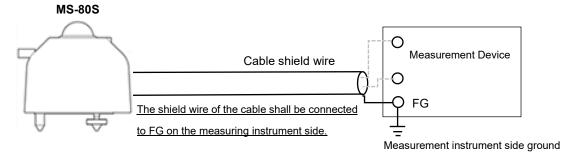
Figure 5-4B. MS-80S ground connection method
