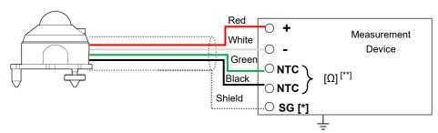
Figure 5-7. How to connect MS-80U
