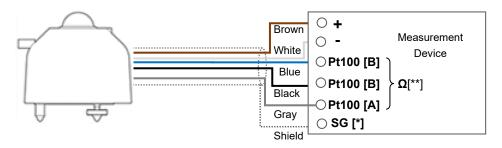
Figure 5-5. How to connect MS-80 (from S/N: S1904615)
