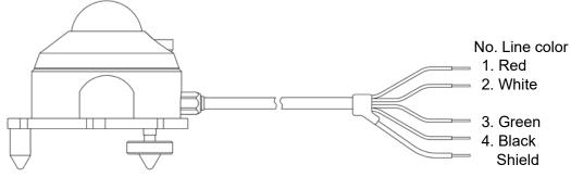
Figure 7-5. Output Cables [MS-80U]
