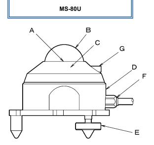
\*The cable can't be removed from the pyranometer Figure 5-2. Pyranometer Parts Name [MS-80U]
