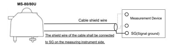
Figure 5-4A. MS-80/80U ground connection method
