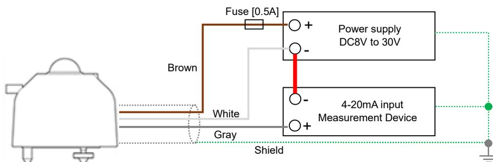
Figure 5-8. How to connect MS-80S (4-20mA output)
