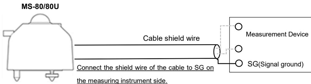
Figure 5-4A. MS-80/80U ground connection method
