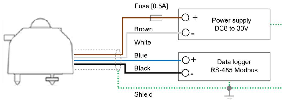
Figure 5-11. How to connect MS-80S (Modbus RS-485)
