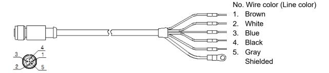
Figure 7-3. Output-Cable [MS-60S]
