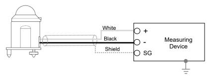
Figure 5-4. How to connect MS-60 (Analog output)
