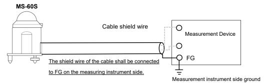
Figure 5-3B. MS-60S shield wire connection method
