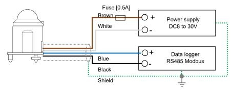
Figure 5-8. How to connect MS-60S (Modbus RTU)
