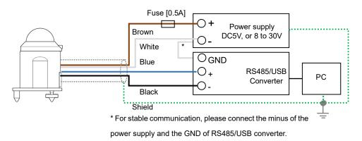
Figure 5-7. How to connect MS-60S (Modbus RTU)
