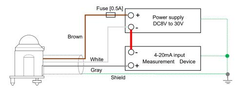
Figure 5-5. How to connect MS-60S (4-20mA output)
