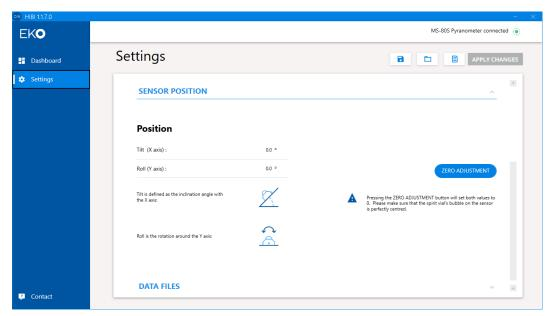
Figure A3-18. Sensor Position setting
