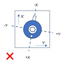
Figure 5-2C Tilt and roll angle not corresponding to reference plane
