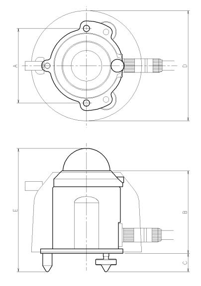
Figure 7-1. External Dimensions [MS-60/60S]
