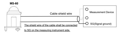
Figure 5-3A. MS-60 shield wire connection method
