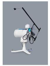
The MS-57SH Pyrheliometer is designed for solar assessment, research, concentrated photovoltaic applications and solar monitoring. Mounted on a sun tracker, the MS-57SH, with its ultra-fast <0.3 response, unique characteristics, S-Series internal diagnostics and superior design, ensure best in class accuracy, speed, and reliability whatever your application.
